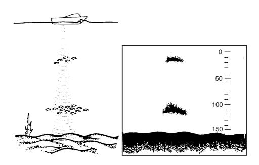
Figure 2-1 Underwater conditions and video sounder display
